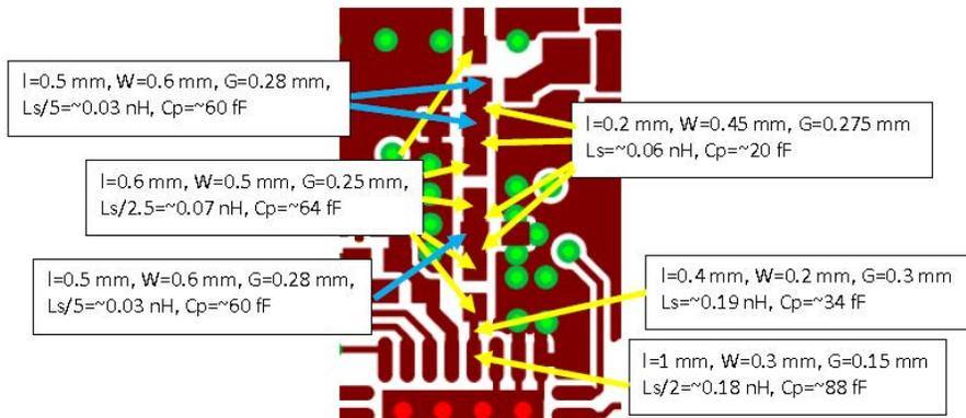
Image from AN930 on Blue Gecko Bluetooth Smart antenna matching
